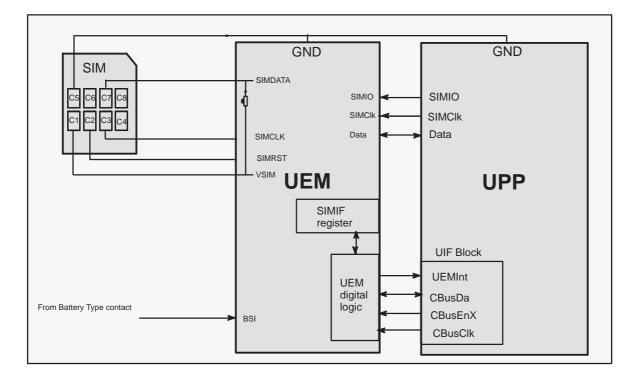
The internal clock frequency from UPP CTSI block is 13 MHz in GSM. Thus to achieve the minimum starting SIMCardClk rate of 3.25 MHz (as is required by the authentication procedure and the duty cycle requirement of between 40% and 60%) then the slowest possible clock supplied to the SIM has to be in the GSM system clock rate of 13/4 MHz.
